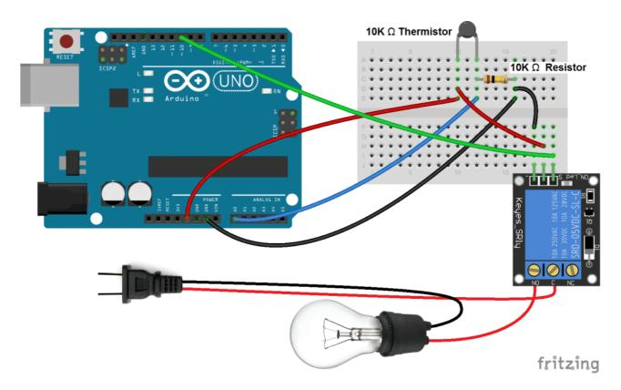
Identify the hot power wire (red wire in the diagram above) in the cord leading to the light bulb and make a cut. Connect the side leading to the light bulb to the NO terminal of the relay, and the side leading to the plug to the C terminal. This way the relay is on the hot side, and current is switched before it reaches the light bulb. It's dangerous to put the relay on the neutral wire, since if the device fails current can still fault to ground when the relay is off.
