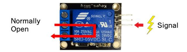
In the normally open configuration, when the relay receives a HIGH signal the 120-240V switch closes and allows current to flow from the C terminal to the NO terminal. A LOW signal deactivates the relay and stops the current. So if you want the HIGH signal to turn ON the relay, use the normally open terminal:
